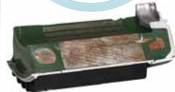
Insulated motor winding cross section
